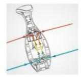
Air cooling system permits to work longer without overheating.
